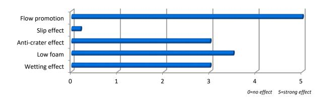
**LNIC**<sup>®</sup>**FLOW 383 S** is modified polyester leveling agents to be used in solvent based coating system. Shows excellent compatibility with most of the resins. It shows the good fast wetting and leveling and strong defoaming performances, It will improve DOI and fullness. it shows good performance in automotive and industrial coating
